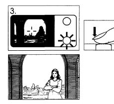
**3.** Reposition your subject in the picture frame while keeping the shutter release button depressed halfway. Then press the shutter release button fully.
